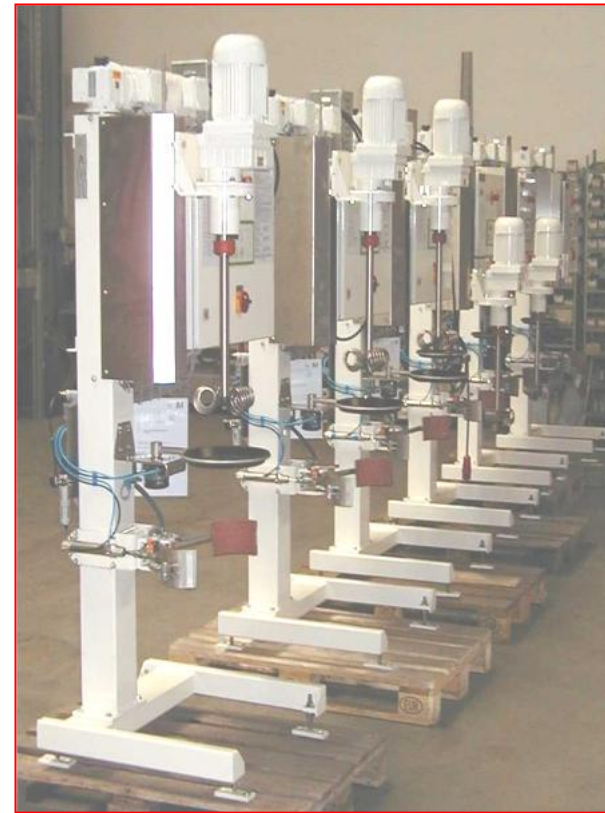
VJ400 VA column agitator for fully automatic operation with PLC control system for serial production
