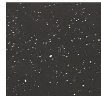
Spattering produced by HEC 6000 product
