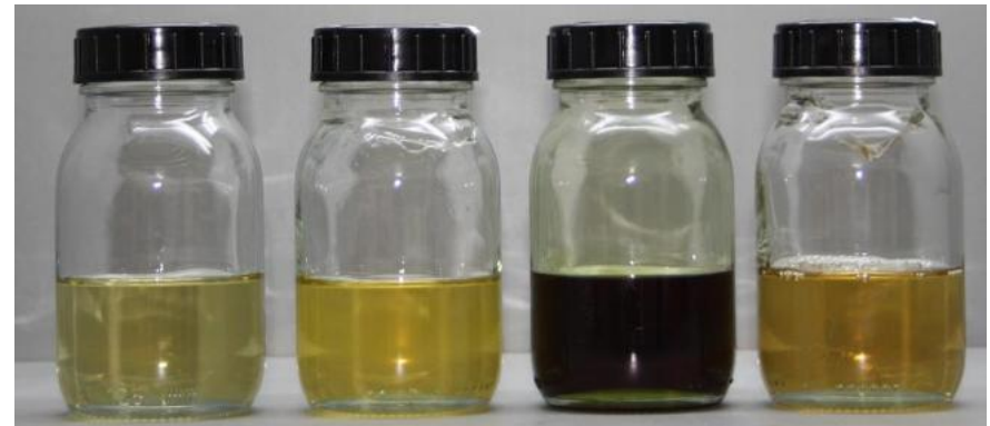
Binder Binder + 0.4% BOC 1310 Binder + 0.5% Competitor, Mn based Binder + 0.1% Borchers® Dry 0411 HS (our accelerated Mn)
