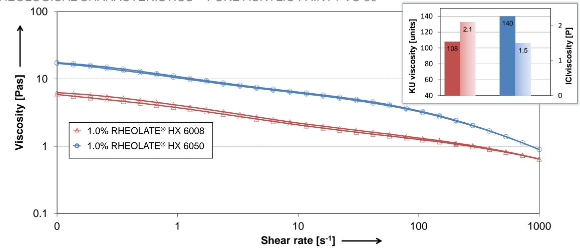
Rheological data determined using the Anton-Paar MCR 300 rheometer, measuring geometry PP 50, at a temperature of 23°C; ICI viscosity indicates the viscosity at high shear rates of 10000 s<sup>-1</sup>; KU describes the Krebs-Stormer viscosity; tested in a pure acrylic pvc 30% paint system; viscosity data of unthickened paint: ICI 0.2 and KU 47
