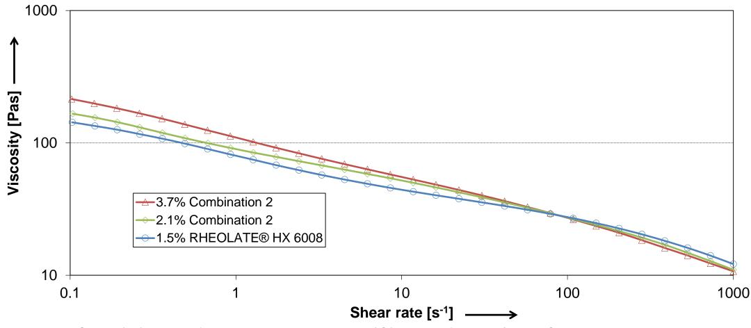
Paint adjusted to a Krebs-Stormer (KU) viscosity of ca. 118 ±1 units <u>and</u> a high-shear (ICI) viscosity of about 3 +/- 0.2 P; ICI viscosity indicates the viscosity at high shear rates of 10000 s<sup>-1</sup>; KU describes the Krebs-Stormer viscosity; tested in a pure acrylic pvc 30% paint system; Rheological data determined using the Anton-Paar MCR 300 rheometer, measuring geometry PP 50, at a temperature of 23°C
