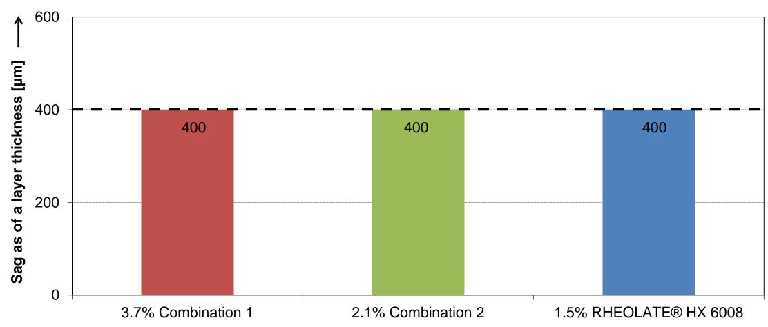
Paint adjusted to a Krebs-Stormer (KU) viscosity of ca. 118 ±1 units <u>and</u> a high-shear (ICI) viscosity of about 3 +/- 0.2 P; ICI viscosity indicates the viscosity at high shear rates of 10000 s<sup>-1</sup>; KU describes the Krebs-Stormer viscosity; tested in a pure acrylic pvc 30% paint system; Sag stability tested using test blade 1000 -100µm; the larger the bar, the better the result
