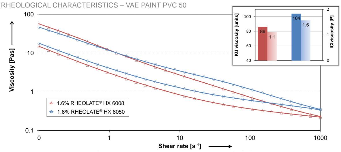
Rheological data determined using the Anton-Paar MCR 300 rheometer, measuring geometry PP 50, at a temperature of 23°C; ICI viscosity indicates viscosity at high shear rates of 10000 s<sup>-1</sup>; KU is the Krebs-Stormer viscosity; tested in a Vinylacetate/Ethylene (VAE) based pvc 50% paint system; viscosity data of unthickened paint: ICI 0.35 and KU 65
