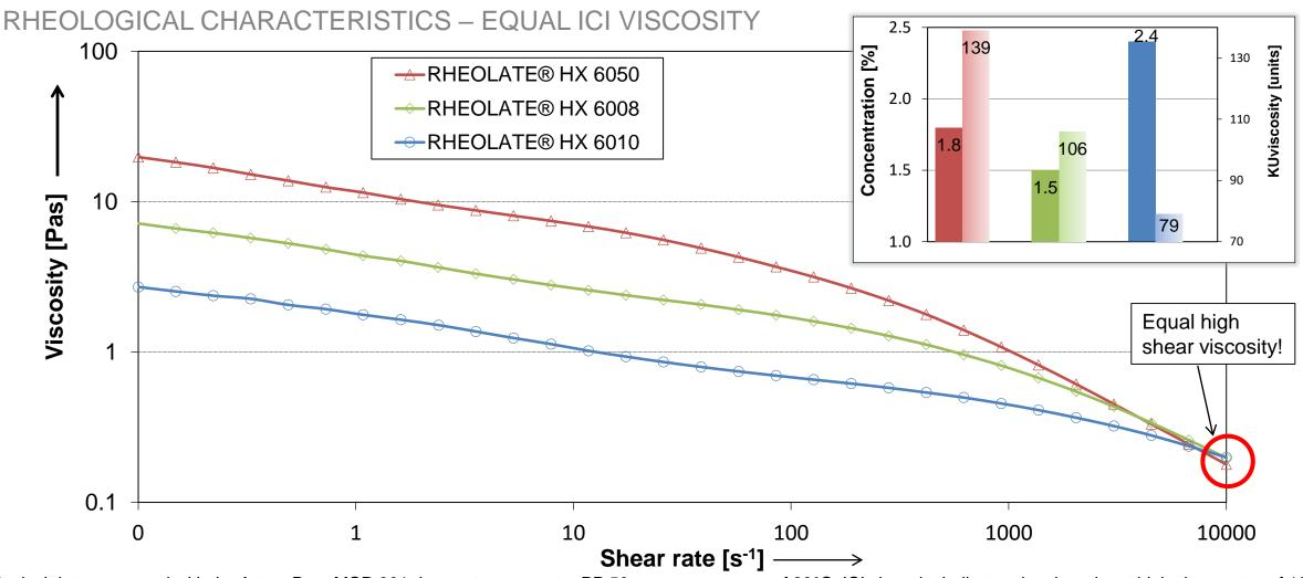
Rheological data measured with the Anton-Paar MCR 301 rheometer, geometry PP 50, at a temperature of 23°C; ICI viscosity indicates the viscosity at high shear rates of 10000 s<sup>-1</sup>; KU describes the Krebs-Stormer viscosity; All samples adjusted to equal ICI viscosity of 2.0 Poise; Pure acrylic pvc 30 paint
