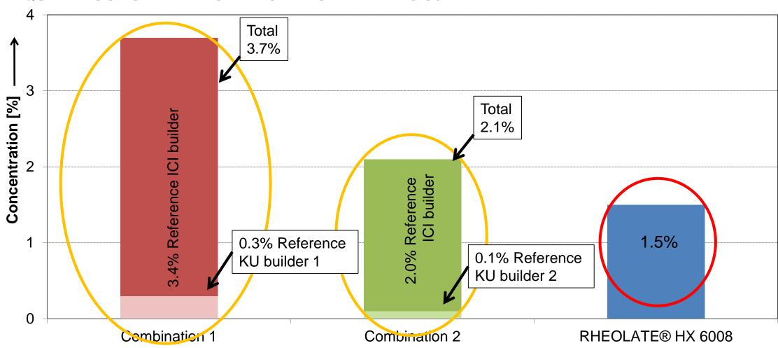
Concentration required to achieve Krebs-Stormer (KU) viscosity of ca. 118 ±1 units <u>and</u> a high-shear (ICI) viscosity of about 3 +/- 0.2 P; ICI viscosity indicates the viscosity at high shear rates of 10000 s<sup>-1</sup>; KU describes the Krebs-Stormer viscosity; tested in a pure acrylic pvc 30% paint system
