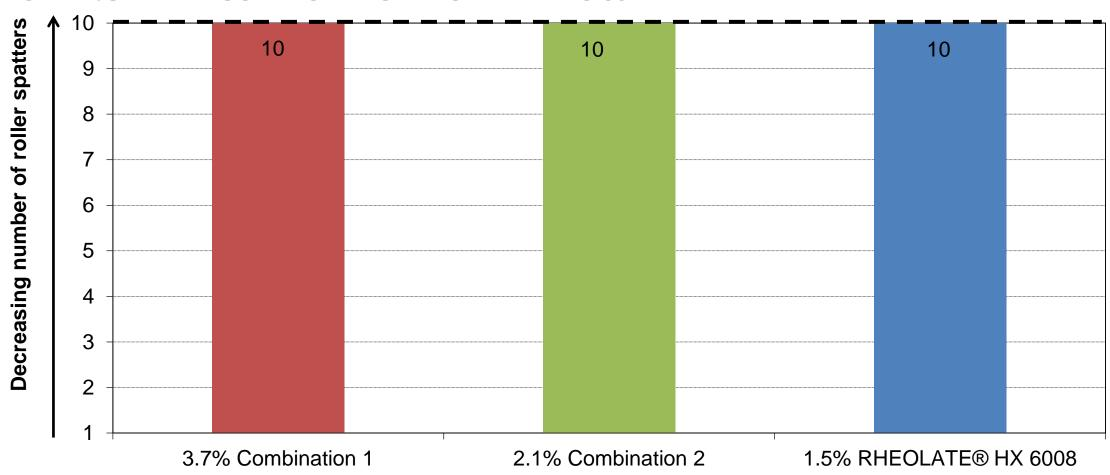
Paint adjusted to a Krebs-Stormer (KU) viscosity of ca. 118 ±1 units <u>and</u> a high-shear (ICI) viscosity of about 3 +/- 0.2 P; ICI viscosity indicates the viscosity at high shear rates of 10000 s<sup>-1</sup>; KU describes the Krebs-Stormer viscosity; tested in a pure acrylic pvc 30% paint system; 40g of paint rolled on vertical wall (10 times up & down); Spatters collected on black chart underneath and judged visually; the larger the bar the better the result
