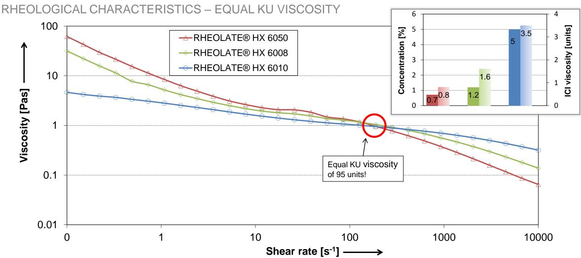
Rheological data measured with the Anton-Paar MCR 301 rheometer, geometry PP 50, at a temperature of 23°C; ICI viscosity indicates the viscosity at high shear rates of 10000 s<sup>-1</sup>; KU describes the Krebs-Stormer viscosity; All samples adjusted to equal KU viscosity of 95 units; Pure acrylic pvc 30 paint
