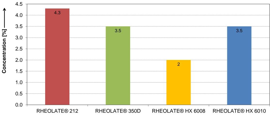
Concentration necessary to achieve equal high-shear (ICI) viscosity of 4.0 units; Rheological data determined at a temperature of 23°C; ICI viscosity indicates the viscosity at high shear rates of 10000 s<sup>-1</sup>; tested in an aqueous PU-alkyd based paint
