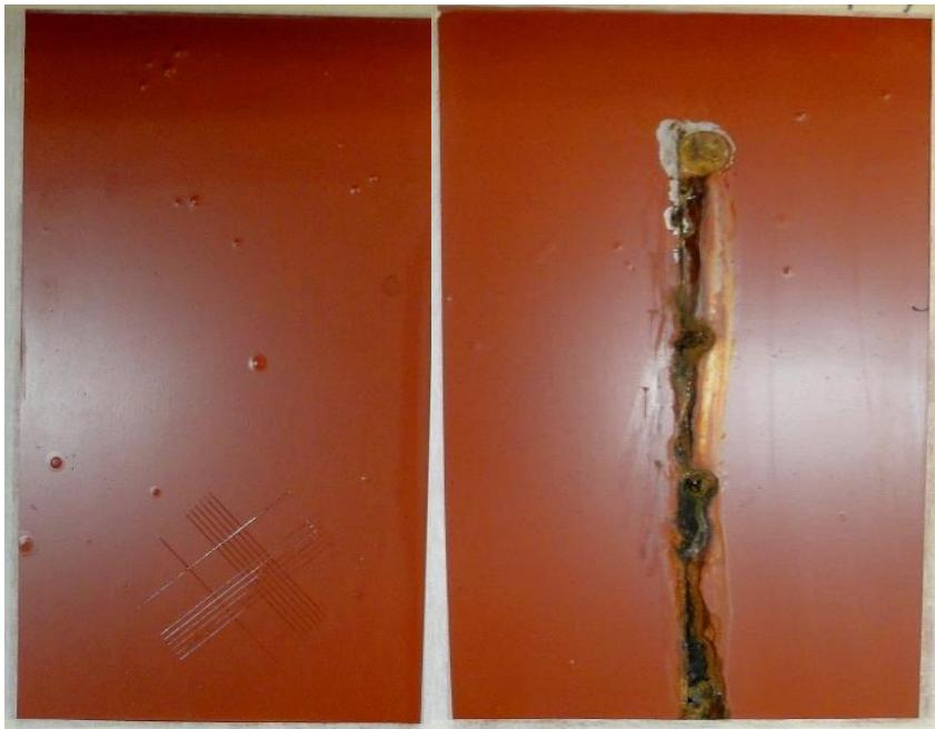
**Test specimen of Urakyd AK429 X-60 and Urathix B3201 60X (AK15050) after 1000 h corrosion test: adhesion, blistering and delamination results are shown.**
